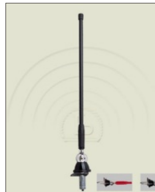
#13-4323 ● Universal roof, front or rear fender mount ● 1 section flexible rubber mast ● Swivel ball base 180° adjustable angle ● Extends to 15" ● Cable: 54"
