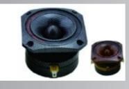
Nominal Impedance: 4--8ohm Power Capacity: 30 RMS W Sensitivity (1w/1m): 106 db Frequency Range: 2KHZ-16KHZ Voice Coil Diameter: 25.4mm Voice coil Material: Ronud copper wire Voice Coil Former: KSV Diaphragm Material: Titanium Housing Material: Plastic Magnet Weight: 7.8Oz Overall Diameter: 80.0mm Overall Depth: 63.0mm Net Weight: 0.5kg
