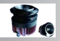
Nominal Impedance: 4--8ohm Power Capacity: 25 RMS W Sensitivity (1w/1m): 102 db Frequency Range: 2KHZ-20KHZ Voice Coil Diameter: 25.4mm Voice coil Material: CCAW Voice Coil Former: KSV Diaphragm Material: Titanium Housing Material: Aluminum Magnet Size: 25\*7 Overall Diameter: 58.0mm Overall Depth: 59.5mm Net Weight: 0.6kg
