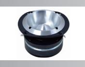
Nominal Impedance: 4--8ohm Power Capacity: 40 RMS W Sensitivity (1w/1m): 106 db Frequency Range: 2KHZ-20KHZ Voice Coil Diameter: 44.4mm Voice coil Material: CCAW Voice Coil Former: KSV
