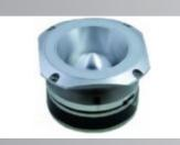
Nominal Impedance: 4--8ohm Power Capacity: 40 RMS W Sensitivity (1w/1m): 105 db Frequency Range: 2KHZ-20KHZ Voice Coil Diameter: 44.4mm Voice coil Material: CCAW Voice Coil Former: KSV Diaphragm Material: Titanium Housing Material: Aluminum Magnet Weight: 11.3Oz Overall Diameter: 100.0mm Overall Depth: 75.0mm Net Weight: 1.5kg
