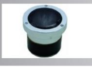
Nominal Impedance: 4--8ohm Power Capacity: 30 RMS W Sensitivity (1w/1m): 106 db Frequency Range: 2KHZ-20KHZ Voice Coil Diameter: 25.4mm Voice coil Material: CCAW Voice Coil Former: KSV Diaphragm Material: Titanium Housing Material: Aluminum Magnet Weight: 15.6Oz Overall Diameter: 89.0mm Overall Depth: 78.0mm Net Weight: 1.4kg
