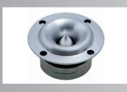
Nominal Impedance: 4--8ohm Power Capacity: 30 RMS W Sensitivity (1w/1m): 106 db Frequency Range: 2KHZ-20KHZ Voice Coil Diameter: 25.4mm Voice coil Material: CCAW Voice Coil Former: KSV Diaphragm Material: Titanium Housing Material: Aluminum Magnet Weight: 5.2Oz Overall Diameter: 100.0mm Overall Depth: 85.0mm Net Weight: 0.6kg
