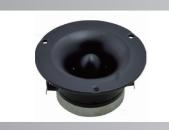
Nominal Impedance: 4--8ohm Power Capacity: 30 RMS W Sensitivity (1w/1m): 105 db Frequency Range: 2KHZ-20KHZ Voice Coil Diameter: 32.4mm Voice coil Material: CCAW Voice Coil Former: KSV Diaphragm Material: Titanium Housing Material: Aluminum Magnet Size: 32\*16\*7 Overall Diameter: 100.5mm Overall Depth: 47.0mm Net Weight: 0.6kg
