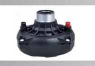
Nominal Impedance: 4--8ohm Power Capacity: 45 RMS W Sensitivity (1w/1m): 105 db Frequency Range: 2KHZ-20KHZ Voice Coil Diameter: 50.8mm Voice coil Material: CCAW Voice Coil Former: KSV
