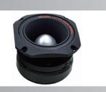
Nominal Impedance: 4--8ohm Power Capacity: 40 RMS W Sensitivity (1w/1m): 102 db Frequency Range: 2KHZ-20KHZ Voice Coil Diameter: 44.4mm Voice coil Material: CCAW Voice Coil Former: KSV
