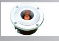
Nominal Impedance: 4--8ohm Power Capacity: 30 RMS W Sensitivity (1w/1m): 109 db Frequency Range: 2KHZ-20KHZ Voice Coil Diameter: 25.4mm Voice coil Material: CCAW Voice Coil Former: KSV Diaphragm Material: Titanium Housing Material: Aluminum Magnet Size: 25\*7 Overall Diameter: 79.0mm Overall Depth: 53.0mm Net Weight: 0.55kg
