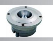
Nominal Impedance: 4–8ohm Power Capacity: 30 RMS W Sensitivity (1w/1m): 109 db Frequency Range: 2KHZ-20KHZ Voice Coil Diameter: 25.4mm Voice coil Material: CCAW Voice Coil Former: KSV Diaphragm Material: Titanium Housing Material: Aluminum Magnet Size: 25\*7 Overall Diameter: 79.0mm Overall Depth: 53.0mm Net Weight: 0.55kg
