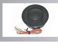
Nominal Impedance: 4--8ohm Power Capacity: 20 RMS W Sensitivity (1w/1m): 90 db Frequency Range: 2KHZ-20KHZ Voice Coil Diameter: 13.28mm Voice coil Material: Round copper wire Voice Coil Former: KSV Diaphragm Material: Ployester Housing Material: Plastic Magnet Size: 12.8\*2 Overall Diameter: 54.5mm Overall Depth: 22.2mm Net Weight: 0.03kg
