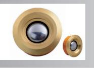
Nominal Impedance: 4--8ohm Power Capacity: 20 RMS W Sensitivity (1w/1m): 90 db Frequency Range: 2KHZ-20KHZ Voice Coil Diameter: 25.4mm Voice coil Material: CCAW Voice Coil Former: KSV
