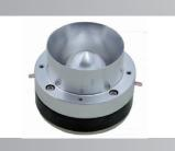
Nominal Impedance: 4--8ohm Power Capacity: 40 RMS W Sensitivity (1w/1m): 106 db Frequency Range: 2KHZ-20KHZ Voice Coil Diameter: 44.4mm Voice coil Material: CCAW Voice Coil Former: KSV
