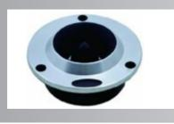
Nominal Impedance: 4--8ohm Power Capacity: 30 RMS W Sensitivity (1w/1m): 106 db Frequency Range: 2KHZ-20KHZ Voice Coil Diameter: 25.4mm Voice coil Material: Ronud copper wire Voice Coil Former: KSV Diaphragm Material: Titanium Housing Material: Aluminum Magnet Weight: 5.2Oz Overall Diameter: 100.0mm Overall Depth: 85mm Net Weight: 0.6kg
