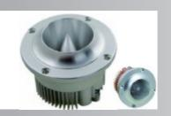
Nominal Impedance: 4--8ohm Power Capacity: 25 RMS W Sensitivity (1w/1m): 102 db Frequency Range: 2KHZ-20KHZ Voice Coil Diameter: 25.4mm Voice coil Material: CCAW Voice Coil Former: KSV Diaphragm Material: Titanium Housing Material: Aluminum Magnet Size: 25\*7 Overall Diameter: 70.0mm Overall Depth: 79.0mm Net Weight: 0.6kg
