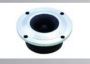
Nominal Impedance: 4--8ohm Power Capacity: 25 RMS W Sensitivity (1w/1m): 102 db Frequency Range: 2KHZ-20KHZ Voice Coil Diameter: 25.4mm Voice coil Material: Ronud copper wire Voice Coil Former: KSV Diaphragm Material: Titanium Housing Material: Aluminum Magnet Weight: 5..2Oz Overall Diameter: 95.0mm Overall Depth: 40.0mm Net Weight: 0.52kg
