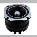
Nominal Impedance: 4--8ohm Power Capacity: 43 RMS W Sensitivity (1w/1m): 110 db Frequency Range: 2KHZ-16KHZ Voice Coil Diameter: 46.0 mm Voice coil Material: Round copper wire Voice Coil Former: KSV
