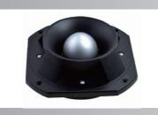
Nominal Impedance: 4--8ohm Power Capacity: 48 RMS W Sensitivity (1w/1m): 105 db Frequency Range: 2KHZ-20KHZ Voice Coil Diameter: 62.0mm Voice coil Material: Round copper wire Voice Coil Former: KSV
