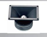
Nominal Impedance: 4--8ohm Power Capacity: 43 RMS W Sensitivity (1w/1m): 100 db Frequency Range: 2KHZ-16KHZ Voice Coil Diameter: 44.4mm Voice coil Material: CCAW Voice Coil Former: KSV
