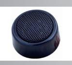
Nominal Impedance: 4--8ohm Power Capacity: 17 RMS W Sensitivity (1w/1m): 90 db Frequency Range: 2KHZ-20KHZ Voice Coil Diameter: 19.4mm Voice coil Material: Round copper wire Voice Coil Former: KSV Diaphragm Material: Silk Housing Material: Plastic Magnet Size: 19\*3 Overall Diameter: 36.2mm Overall Depth: 24.3mm Net Weight: 0.03kg
