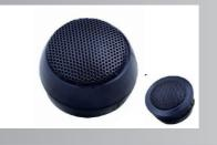
Nominal Impedance: 4--8ohm Power Capacity: 20 RMS W Sensitivity (1w/1m): 90 db Frequency Range: 2KHZ-20KHZ Voice Coil Diameter: 25.4mm Voice coil Material: Round copper wire Voice Coil Former: KSV Diaphragm Material: Silk Housing Material: Plastic Magnet Size: 25\*3 Overall Diameter: 47.0mm Overall Depth: 30.5mm Net Weight: 0.07kg
