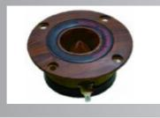
Nominal Impedance: 4--8ohm Power Capacity: 30 RMS W Sensitivity (1w/1m): 106 db Frequency Range: 2KHZ-16KHZ Voice Coil Diameter: 25.4mm Voice coil Material: Ronud copper wire Voice Coil Former: KSV Diaphragm Material: Titanium Housing Material: Plastic Magnet Weight: 5.2Oz Overall Diameter: 97.0mm Overall Depth: 45.0mm Net Weight: 0.4kg
