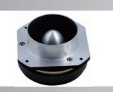
Nominal Impedance: 4--8ohm Power Capacity: 50 RMS W Sensitivity (1w/1m): 110 db Frequency Range: 2KHZ-20KHZ Voice Coil Diameter: 72.0 mm Voice coil Material: CCAW Voice Coil Former: KSV Diaphragm Material: Titanium Housing Material: Aluminum Magnet Weight:45.5 Oz Overall Diameter: 155.0mm Overall Depth: 77.0mm Net Weight: 5.8 kg
