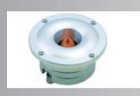
Nominal Impedance: 4--8ohm Power Capacity: 30 RMS W Sensitivity (1w/1m): 110 db Frequency Range: 2KHZ-20KHZ Voice Coil Diameter: 25.4mm Voice coil Material: CCAW
