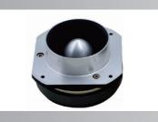
Nominal Impedance: 4–8ohm Power Capacity: 40 RMS W Sensitivity (1w/1m): 102 db Frequency Range: 2KHZ-20KHZ Voice Coil Diameter: 44.4mm Voice coil Material: CCAW Voice Coil Former: KSV Diaphragm Material: Titanium Housing Material: Aluminum Magnet Size: 17.3 Oz Overall Diameter: 110.0mm Overall Depth: 75.0mm Net Weight: 2.2kg
