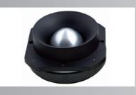
Nominal Impedance: 4--8ohm Power Capacity: 50 RMS W Sensitivity (1w/1m): 110 db Frequency Range: 2KHZ-20KHZ Voice Coil Diameter: 72.0 mm Voice coil Material: CCAW Voice Coil Former: KSV
