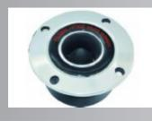
Nominal Impedance: 4--8ohm Power Capacity: 30 RMS W Sensitivity (1w/1m): 103 db Frequency Range: 2KHZ-20KHZ Voice Coil Diameter: 25.4mm Voice coil Material: Ronud copper wire Voice Coil Former: KSV Diaphragm Material: Titanium Housing Material: Aluminum Magnet Weight: 5.2 Oz Overall Diameter: 97.0mm Overall Depth: 45.0mm Net Weight: 0.4kg
