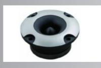
Nominal Impedance: 4--8ohm Power Capacity: 30 RMS W Sensitivity (1w/1m): 106 db Frequency Range: 2KHZ-20KHZ Voice Coil Diameter: 25.4mm Voice coil Material: Ronud copper wire Voice Coil Former: KSV Diaphragm Material: Titanium Housing Material: Aluminum Magnet Weight: 5..2Oz Overall Diameter: 100.0mm Overall Depth: 85.0mm Net Weight: 0.6kg
