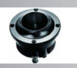
Nominal Impedance: 4--8ohm Power Capacity: 25 RMS W Sensitivity (1w/1m): 102 db Frequency Range: 2KHZ-20KHZ Voice Coil Diameter: 25.4mm Voice coil Material: CCAW Voice Coil Former: KSV Diaphragm Material: Titanium Housing Material: Aluminum Magnet Size: 25\*7 Overall Diameter: 70.0mm Overall Depth: 79.0mm Net Weight: 0.6kg
