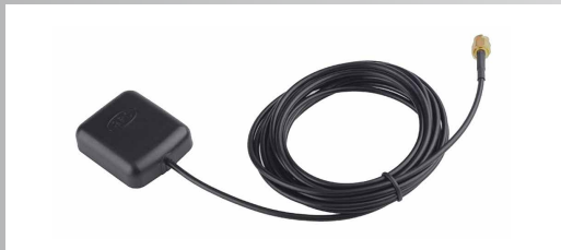
Description GPS&GLONASS Antenna Size: 46*39*13±2mm Weight: <100gram Connector: MCX Male Cable: RG174 1.5 meter Center Frequency: 1575.42/1605MHz V.S.W.R: <1.5 Impedance: 50Ω Supply Voltage: 2.2-5V DC
