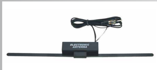
Description Frequency: FM 76-110Mhz AM525-1700Khz Gain:15dBi±3dBi Impedance: 75ohm Voltage: 10-14V Cable length: 2300mm Whip length: 13" Connector: AUDIO Stick install
