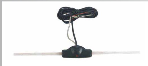
Description Frequency: FM 76-110Mhz AM525-1700Khz Gain:15dBi±3dBi Impedance: 75ohm Voltage: 10-14V Cable length: 2300mm Whip length: 11" Connector: AUDIO Stick install
