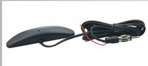
Description Frequency: FM 76-110Mhz AM525-1700Khz Gain:15dBi±3dBi Impedance: 75ohm Voltage: 10-14V Cable length: 2300mm Whip length: 3" Connector: AUDIO Stick install
