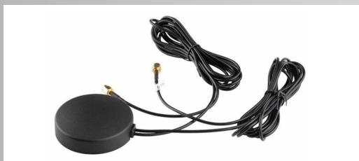
Description GPS+ 4G Antenna Electrical Specifications Frequency Range: 698-2700/MHz 1575.42±5MHz Gain Polarization:≥3dB 27dB V.S.W.R: ≤2.5 Input Connector:SMA Male,SMA Female Mechanical Specifications Dimensions of Antenna: 72.5*21±2mm Cable length: 2m Weight: 93.8gram
